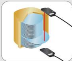
Detection of wafer extending from cassette
