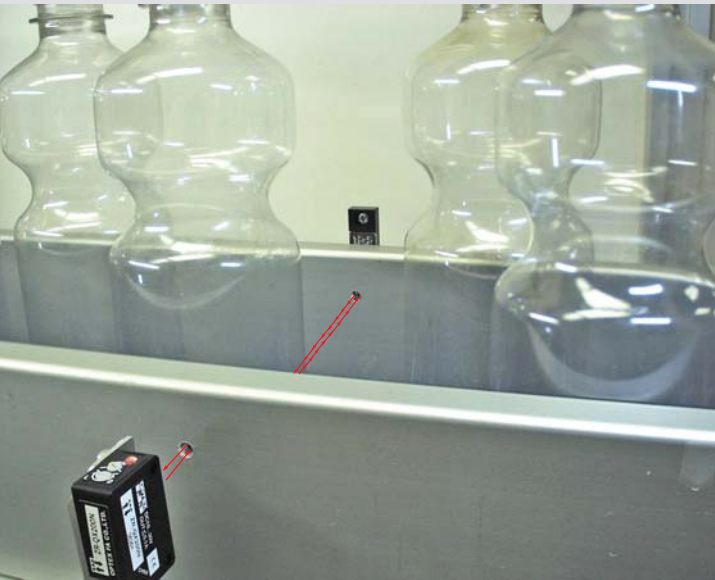
The ZR-QX is designed for transparent object detection. Because the sensor has no dead zone, bottles can be detected regardless of the position on the belt.
