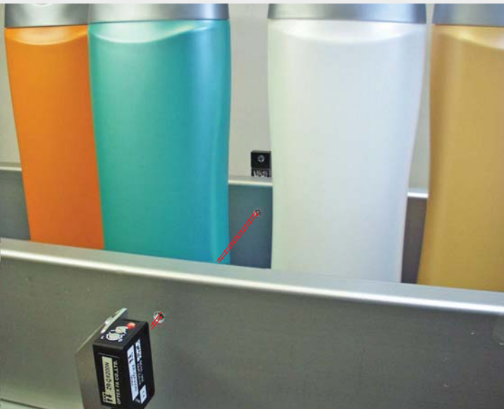
The ZR-X type is designed for non transparent detection. Because the sensor has a coaxial beam, it is ideal for applications requiring the sensor to look through a small slot or opening.
