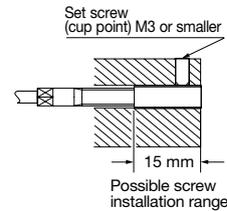
Mounting heat resistant joint fibers (NF-TH12/-TH13/-TH14/-TH15/-TH16)
