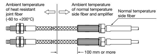
**Mounting narrow view/wafer mapping fibers (NF-TG01/-TG02/-TG03/-TG04)**
