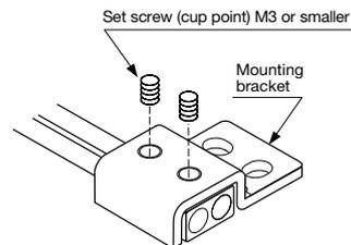
**Mounting through-beam type screen fibers (NF-TZ07/-TZ08/-TZ09/-TZ10)**
