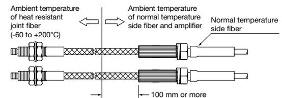
**Mounting narrow view/wafer mapping fibers (NF-TG01/-TG02/-TG03/-TG04)**
