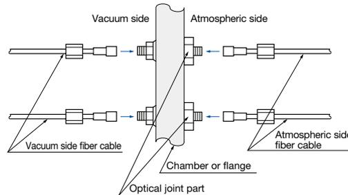
Leakage amount:  $1.33 \times 10^{-10}$  Pa·m<sup>3</sup>/s [He] or less
