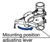
(Note 1): Sensitivity settings must be reconfigured after readjusting the mounting position.
