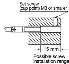
Mounting heat resistant joint fibers (NF-TH12/-TH13/-TH14/-TH15/-TH16)
