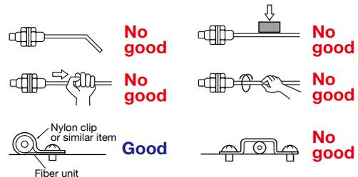
3. Do not apply excessive torque to the sensor head or use tools that do not match the nuts.
