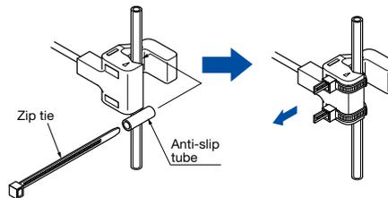
When additional zip ties are necessary, please use zip ties with a thickness 2.5 mm or smaller as shown by (A) in the diagram below.
