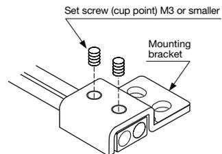
**Mounting through-beam type screen fibers (NF-TZ07/-TZ08/-TZ09/-TZ10)**
