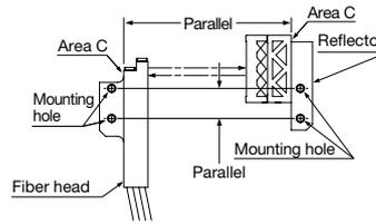
**Mounting liquid leakage detection fibers (NF-DW02)**
