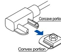
**Mounting pipe-mounted liquid level detection fibers (NF-TF01)**
