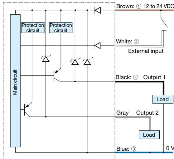
\* Control output 2 (gray) is equipped only for dual-output types. In addition, power supply wires (brown/blue) are not equipped for inter-connection slave units.
