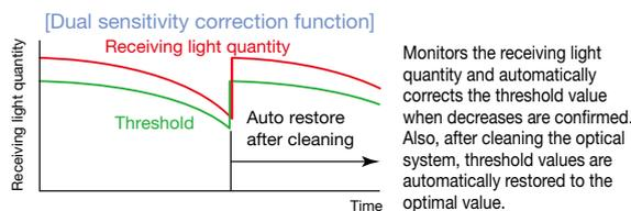
Monitors the receiving light quantity and automatically corrects the threshold value when decreases are confirmed. Also, after cleaning the optical system, threshold values are automatically restored to the optimal value.
