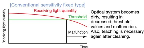
Optical system becomes dirty, resulting in decreased threshold values and malfunction. Also, teaching is necessary again after cleaning.
