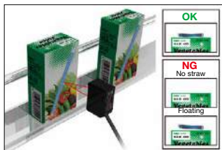
Detecting straws and float (Output 1: ON with no straw; Output 2: ON when floating)
