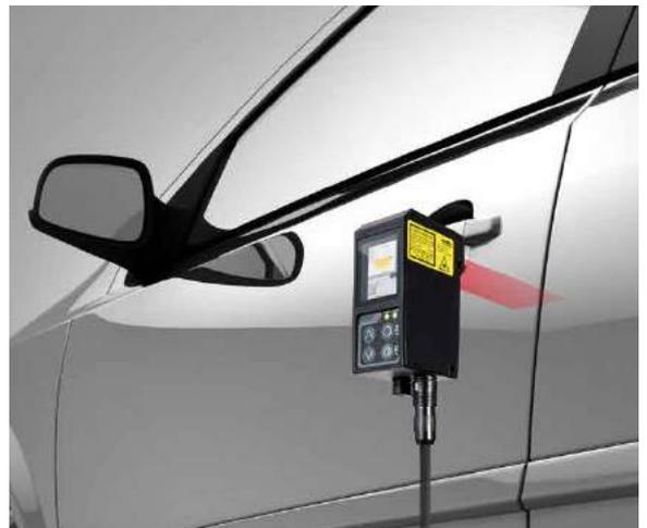
In order to confirm accuracy when installing doors on vehicles, non-contact measurements are performed quickly using the gaps and height differences between the doors and vehicle body.
